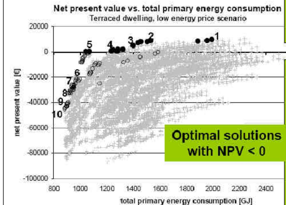
1.  $U = 0.36 \text{W/m}^2\text{K}$  (K30) + HE-boiler + natural ventilation
